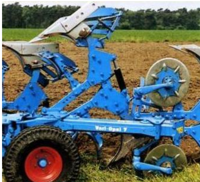
Obr. 11 Hydraulická poistka Hydrix ( http://www.ernest-de.co.uk/images/SPECIALOFFERS1/Lemken%20Plough.jpg )
