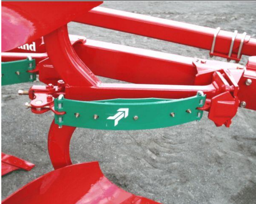
Obr.č.9 Auto – Reset systém Kverneland.
