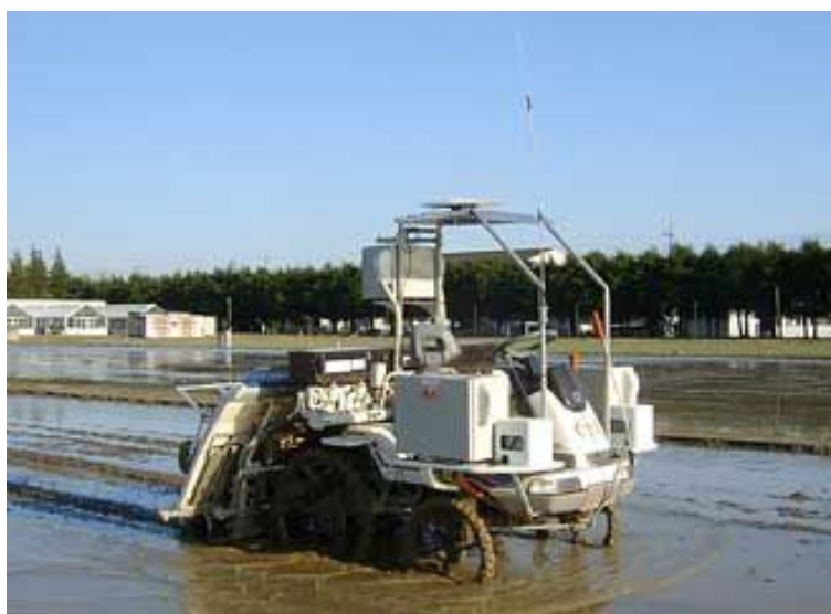
Obr. 16 Rice-planting robot (Japan Echo Inc.2005)
