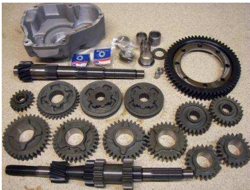
Obr. 14 Ozubené kolesá prevodovky, hriadele
