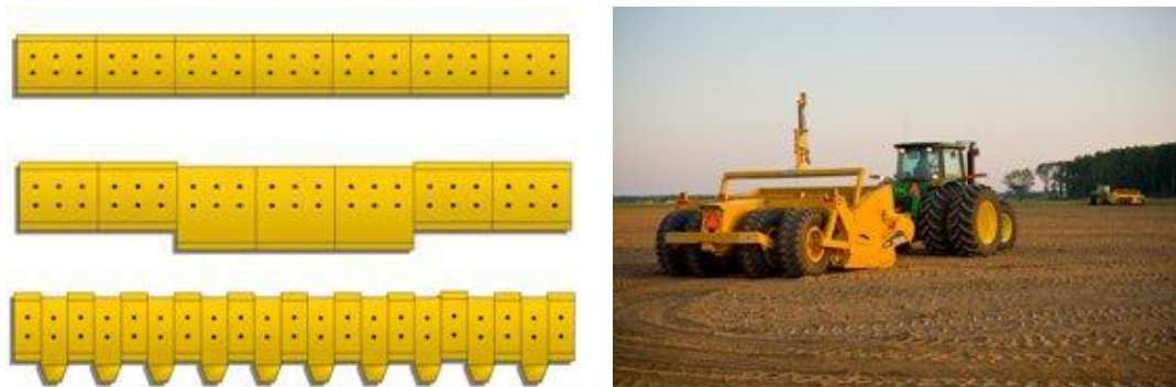
Obr. 19 Scraper John Deere, nože na scraper (Scraper 1512E, 2010)
