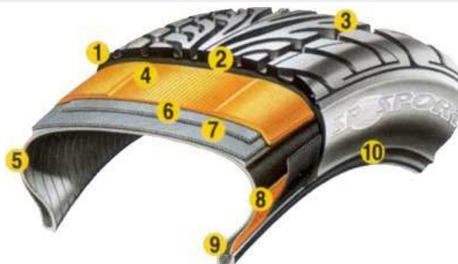
Obr.3 Prierez pneumatikou(Dunlop SP Sport 9000)
