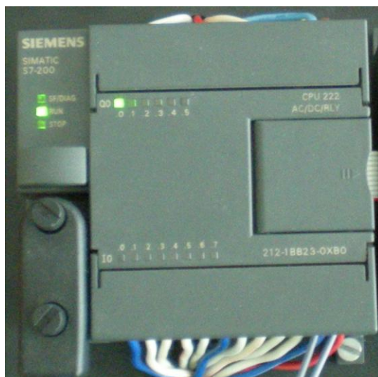
Obr. 22 Simatic S7-200 s CPU 222
